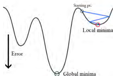
Figure 5: Hill Climbing in the parameter space (Gradient Descent)
